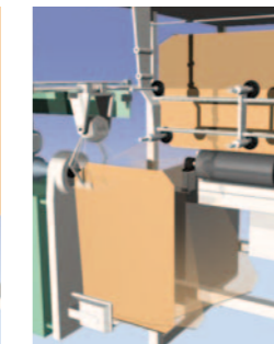
After turning it 90°, the placer sets the bag onto the nozzle.
