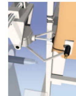
While clamping the bag, the placer opens the valve.
